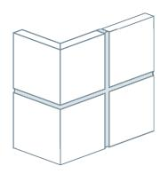
Barrier systems are designed to be completely sealed against moisture intrusion. This is accomplished by utilizing a silicone sealant at each joint to unify the entire system against the elements. (pages 12,36)
